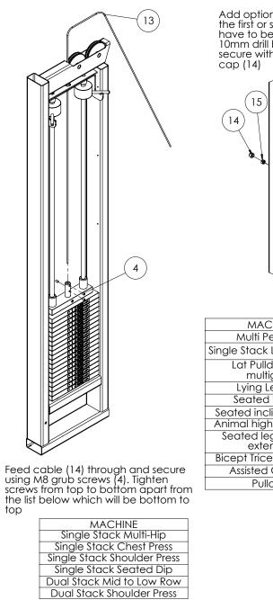
Add optional M10 x 110 bolt (16) to the first or second plate. The plate will have to be drilled through with a 10mm drill bit. See list below secure with nylon nut (15) and end 16 ´14` MACHINE BOLT PLATE Multi Pec/Delt Single Stack Lat Pulldown 1 Lat Pulldown for 1 multigyms Lying Leg Curl Seated leg curl Seated incline lat raise Animal high Pulley Row Seated leg curl/ leg 1 extension Bicept Tricep Machine Assisted Chin Dip 2 Pullover 2 DWG NO. A4 Weight Stack Assembly - Custo
